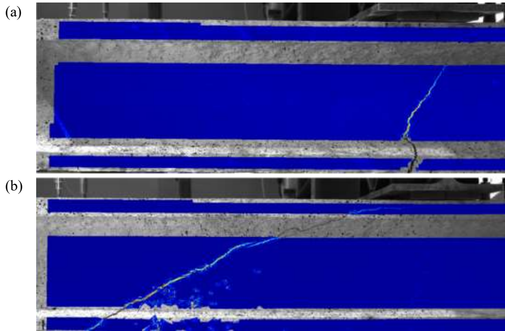
Figure 8: Crack pattern examples for (a) Bending failure of element ID02; (b) Shear failure of element ID04
