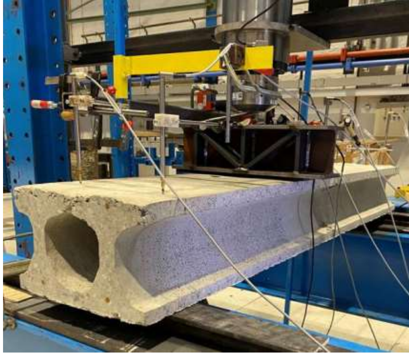
Figure 6: Static test set-up of cut-out element
