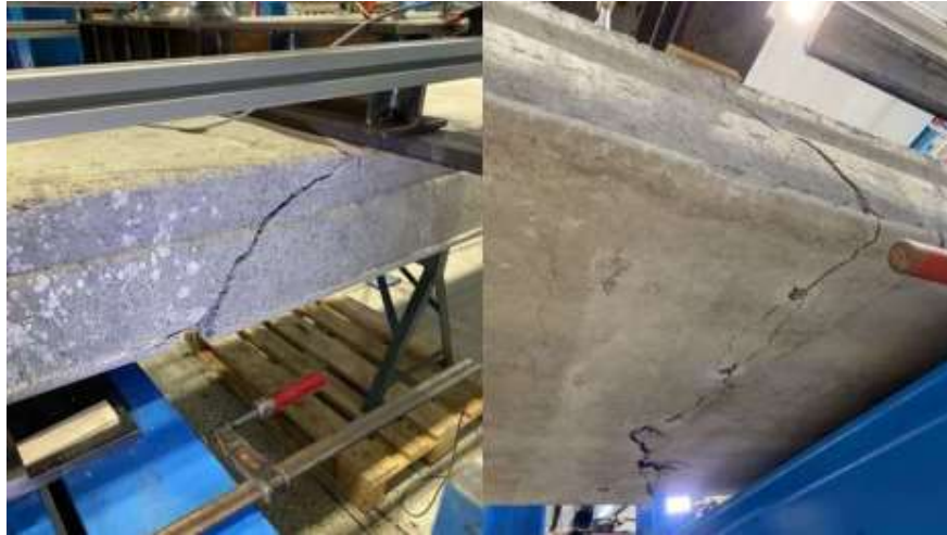
Figure 4: Observed cracking after failure shear failure of HC element testing
