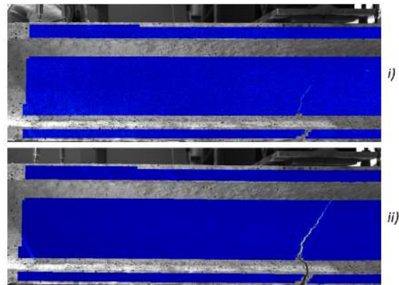
b) Strains recorded by DIC illustrating cracking and moment failure occurring in HD01(upper) and HD02.
