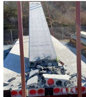
d) Tensile damage viewed from the bottom side of impactor
