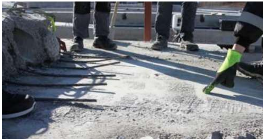
c) Tensile damage viewed from the top side of the floor slab (symmetric half)
